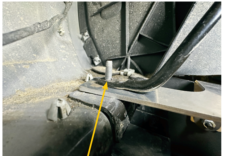
5. Reinstall the factory screw through bracket into fender support rod.
