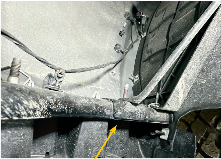
3. Remove 1 factory screw from underside of body.
