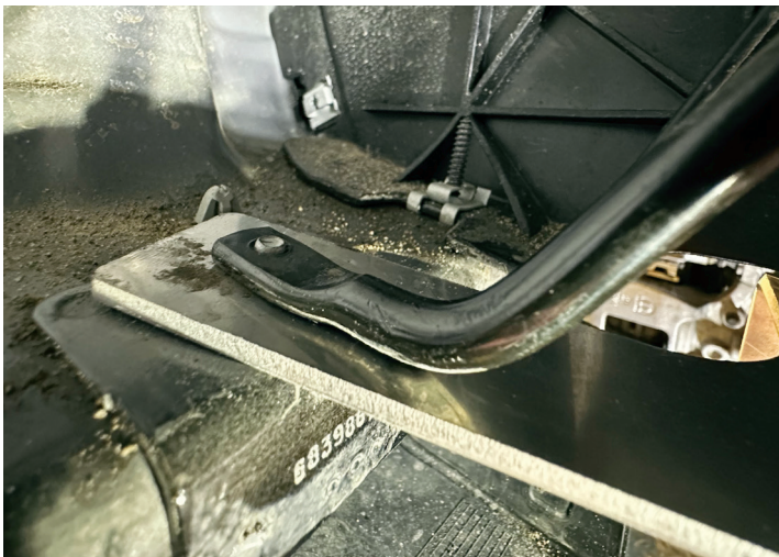
4. Sandwich the bracket between the body and the fender support rod.
