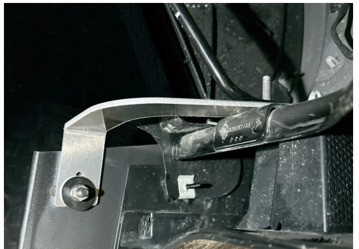
5. Reinstall the factory screw through bracket into fender support rod.
